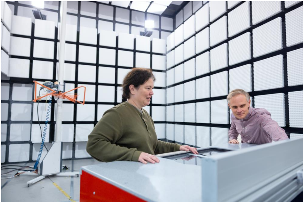
EMC-test in semi-anechoic chambers from 9 kHz to 40 GHz.
