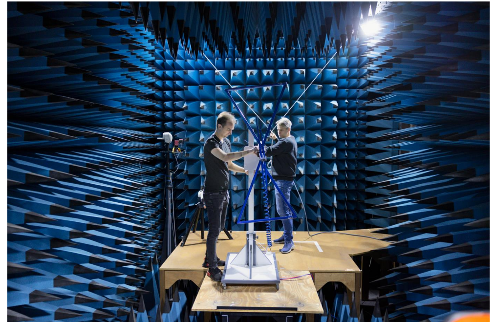
Radio measurements in fully-anechoic chamber 9 kHz to 220 GHz.
