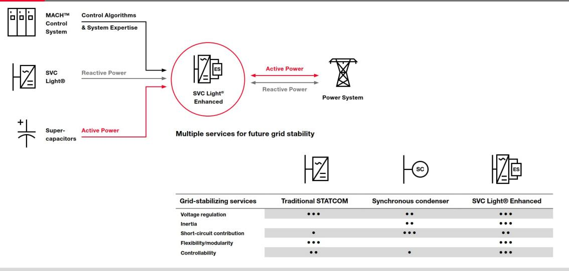
All-in-one solution providing both active and reactive power
