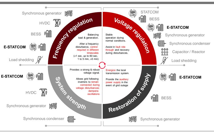
A novel **Hybrid E-STATCOM** design could combine both storage types to leverage their respective advantages
