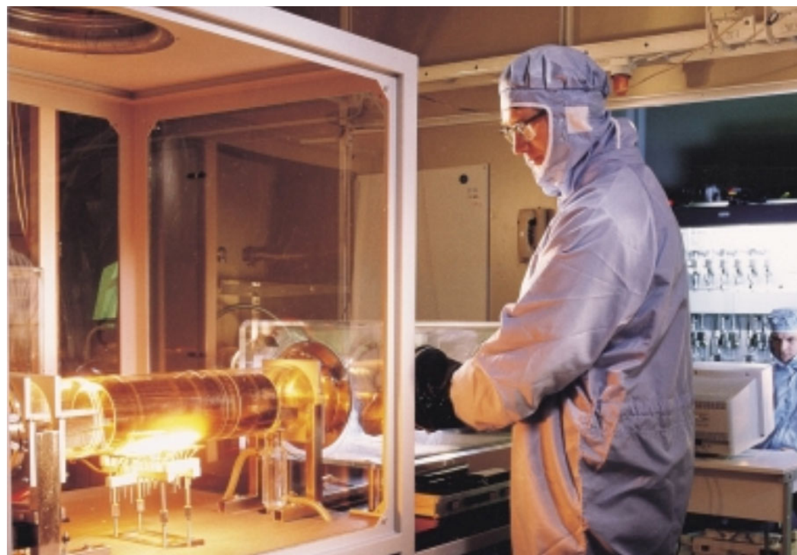
Dr Nils Nordell monitoring the process at IMC in the very first SiC CVD system (1994)
