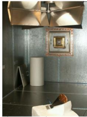
Shielding effectiveness measurements according to IEEE-STD-299, principle.
