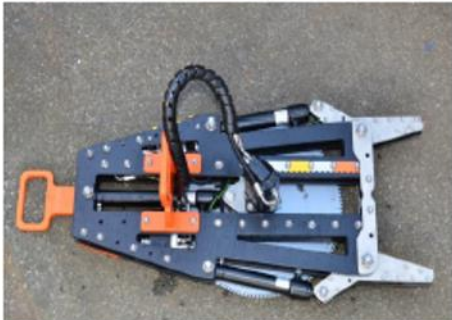
Circular Saw 200mm OD, 120kg
