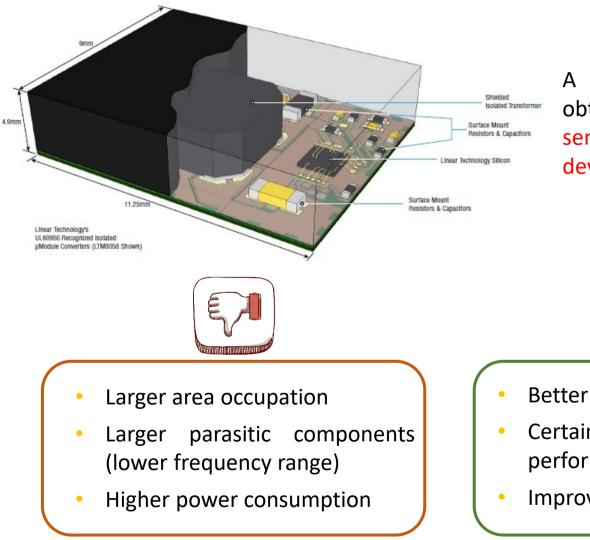
A micromodule can be also obtained by joining a chip level sensor with a discrete level active device and passives.
