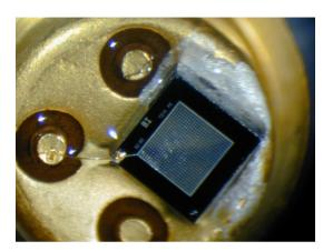
*SiPMs structure*: series combination of an avalanche photodiode (APD or SPAD) with a quenching resistor.
