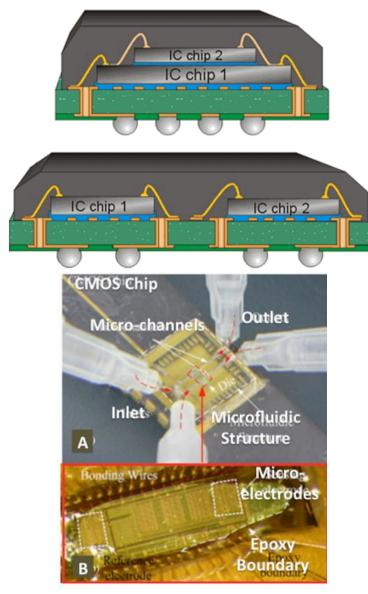
In **micromodule** approach the sensors and the electronic interface circuits are realized on different chips. They are included in the same package or mounted on the same substrate. Interconnections between the sensor and the electronic interface circuit chip can be realized with bonding wires or with other techniques, such as flip-chip or wafer bonding.
