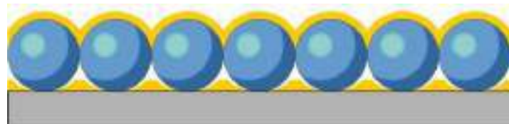
Thin Au layer deposited over the nanobeads array
