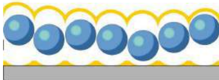
Nanobeads stripping for releasing the metal nanotriangles
