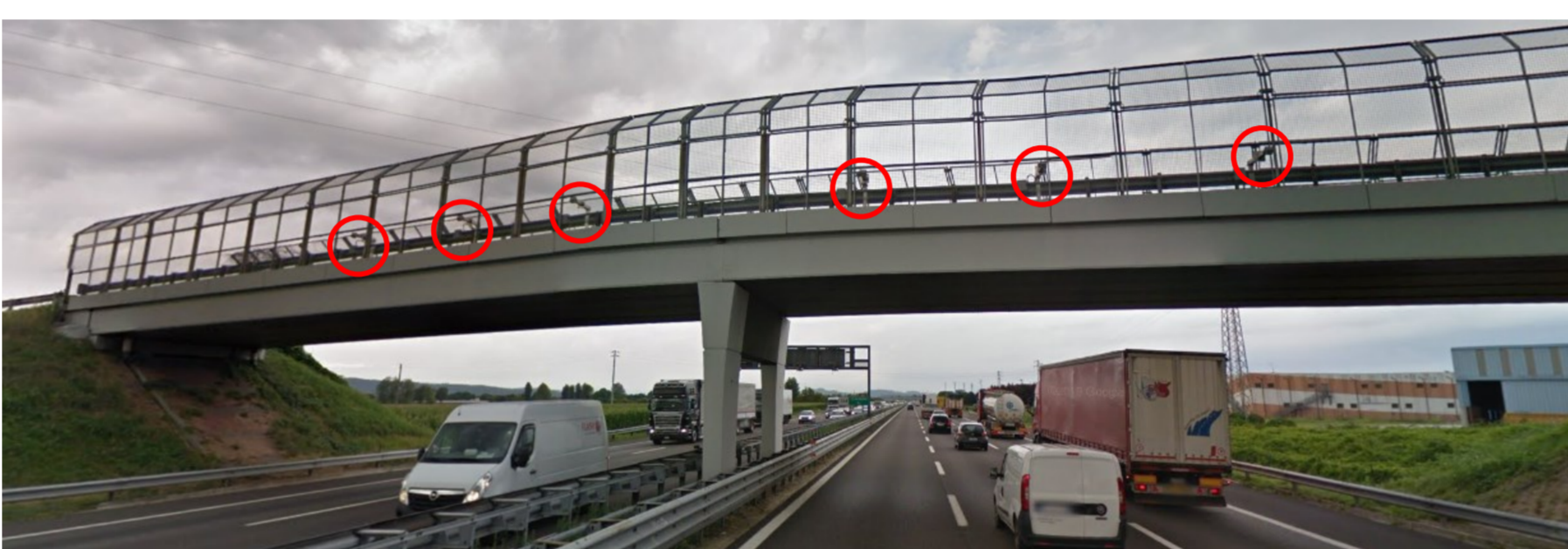
Figure 4. Data collection setup. One radar was positioned above each lane of the cross-section
