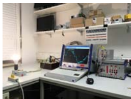
Laboratory measurement of heating due to supraharmonics
